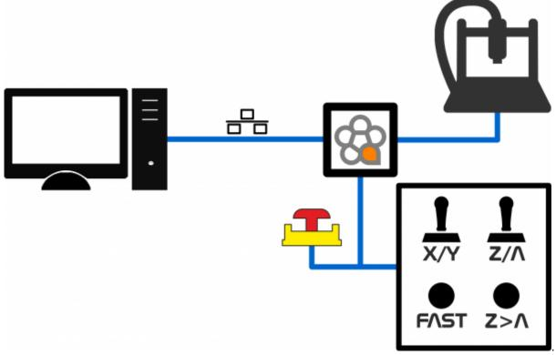
In addition an MPG device can be set up for control of override (feed, rapid, jog or spindle). In this case the value of the "Controller type" parameter must be set to "Dual Joystick".
