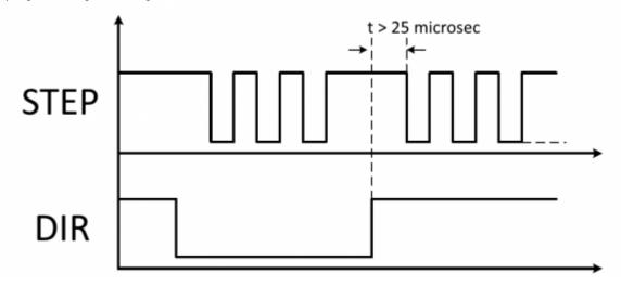
The 25 microsecond time can be configured in the RosettaCNC software.
