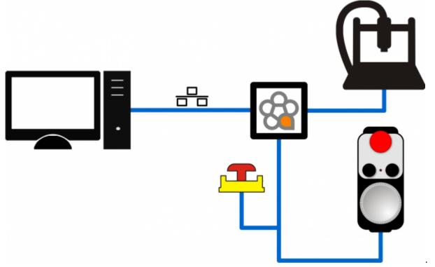
In addition to the flyer, an MPG device for override control can be set up near the machine (feed , rapid, jog or spindle). In this case, the value of the "Controller type" parameter must be set to "HandWheel A".
