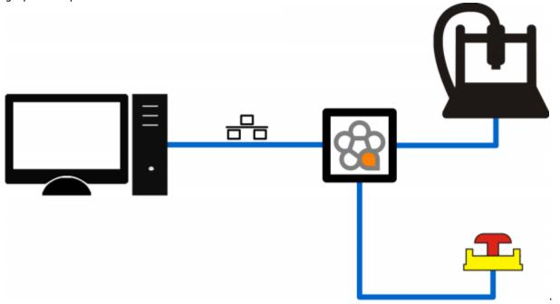
On the machine side only the ESTOP emergency button will be present (and possibly the reset button). In addition, MPG devices for override control (up to two devices) can be set up. In this case the value of the "Controller type" parameter is not significant.
