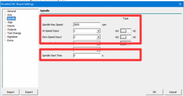
If the inputs are configured then the value in the start time parameter always indicates the minimum wait time although the logic level of the input does not require a wait.
