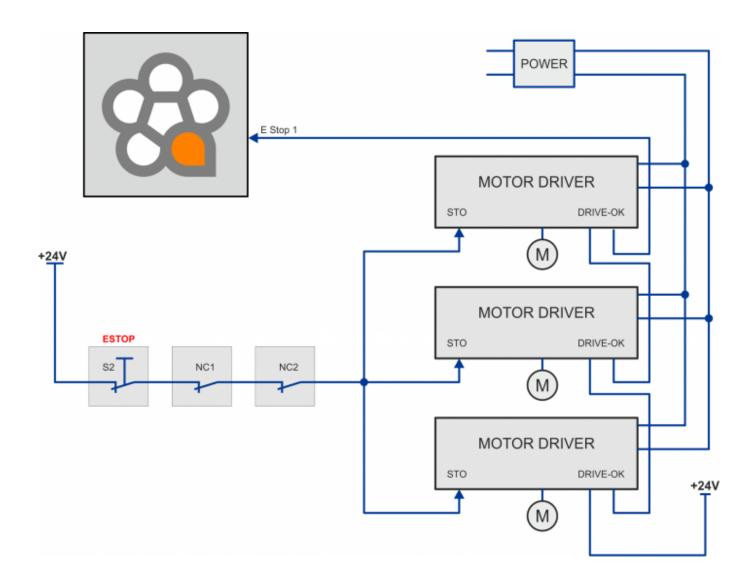
In the below picture, is used a safety device Pilz model PNOZ X7. The emergency button, and possibly other alarm signals (safety barriers, crankcase opening, etc.) must be connected to the input circuits. An output must be connected to the EST1 input of RosettaCNC Board And in series also the drive ok outputs. The other exit of the safety module must be used to stop power to drives.
