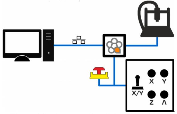
In addition, an MPG device can be set up to control the override (feed, rapid, jog or spindle) . In this case the value of the "Controller type" parameter must be set to "Single Joystick".
