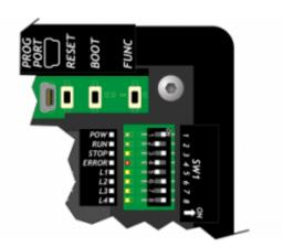
Green Led POW, indicates that the device is powered. Green Led RUN, indicates that the device is working. Yellow Led STOP, indicates that the device is in a stop state
